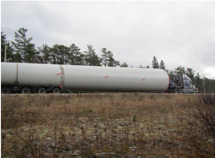
Equipment Delivery. Turbine components including the tower, blades and nacelle are delivered to site.
